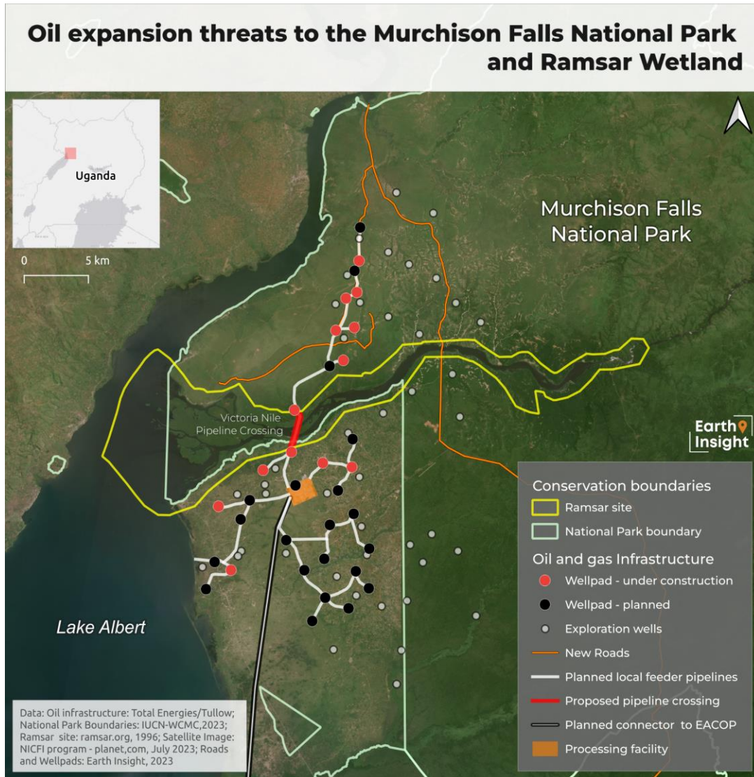
A map showing oil infrastructure affecting a Ramsar wetland and other areas in MFNP
